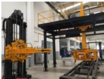
CUBER AND BLOCK TURNING SYSTEM
